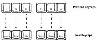
Step 5: Once each keycap is in place, firmly press down on each of the keycaps one at a time to properly secure.
